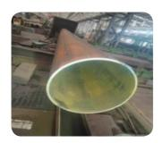
Exhibiting high strength, toughness, a low yield ratio, and a large uniform elongation, this steel fully meets seismic-fault pipeline demands. Produced in small batches and approved by user UOE pipe evaluations, the Company pioneered hot rolling line production of large deformation-resistant pipeline steel, filling an industry gap and supporting national energy pipeline expansion with notable economic and social advantages.
